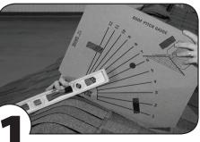
To determine roof pitch, place gauge on peak of roof as shown. Position straight edge as shown. Read roof pitch from printed gauge parallel to bottom of straight edge.
