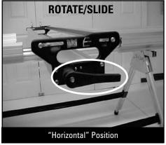
When the handle is in the "horizontal" position, the Boom can move freely while still attached to the saw table base.
