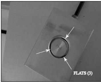
1) The locking block is preset at the factory. If the handle is difficult to turn, remove the boom and inspect the cam shaft and locking block to be certain they are clean and properly lubricated. Rotate the Lock Block 180 degrees and mount the boom. If the handle is still difficult to turn, proceed to step 2.
