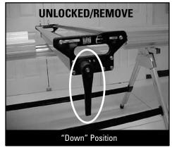
When the handle is in the "down" position, the Boom can be put on or taken off of the table.
