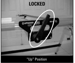
When the handle is in the "up" position, the Boom is locked. The boom must be locked before using the circular saw.
