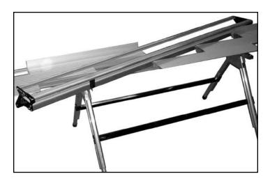
Follow Steps 1-3 of "Using the ProTrax Multi-Angle Saw Table: Angle Cutting" (page 7) or "Using the ProTrax Multi-Angle Saw Table: Cutting 3/12 Pitch" (page 8). The MaxTrax has Deck Extenders that need to be against the Boom when cutting. Slide the Deck Extenders up to the Boom as shown in the figure at right.
