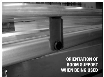
Since the Boom of the MaxTrax is 8 feet long, cutting an angle allows the Boom to flex. Remove the Boom Support from the top of the Boom and install it on the operator side. See figures at left.
