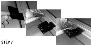
The right hand saw track will stop the saw from kicking up. For added safety, attach the saw keeper to the front of the saw.
