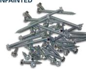
Made of zinc plated steel. Needle point with twin lead thread. Slotted head with ¼-inch indented hex. Larger tub quantities available upon request.
