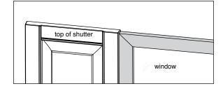
Four fastener application for shutters shorter than 55" Six fastener application for shutters longer than 55"
