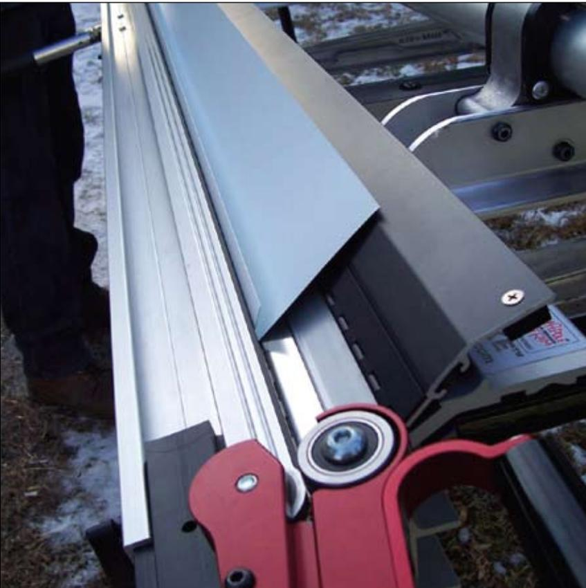
**Hemming** - Lock brake after inserting to desired depth. Bend to the max. Remove. Re-lock brake. Insert between stainless edge and rubber strip. Pull on handle to crush angle flat.
