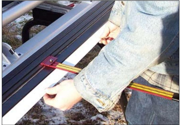
**Transporting your brake** - aside from clamping scrap materials in your brake to prevent internal scratching, it is a good idea to remove your splitter while traveling. This is accomplished by pulling the spring loaded pin and sliding the splitter off the brake splitter track.
