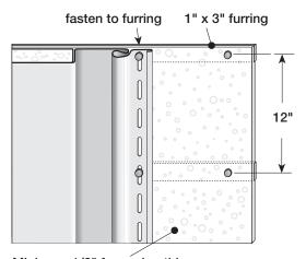
Minimum 1/2" foam sheathing applied on top of strips
