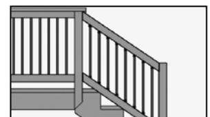
Step 10: Make sure connectors are properly aligned, apply silicone caulk to each stair connector, and assemble the top and bottom rails with the balusters. Then attach full rail section between the stair rail posts.
