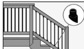
Step 7: Stair rails and balusters can present an installation challenge. DecoRators angled stair rail connectors (sold separately) create a snug and accurate baluster fit for stair angles ranging from 30 to 35 degrees. Cut top and bottom stair rails at the proper angle. Lay top and bottom 2x4 rails alongside the posts and mark.
