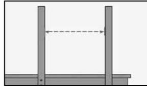
Step 1: Measure railing opening from post to post to determine the length of each baluster rail section.
