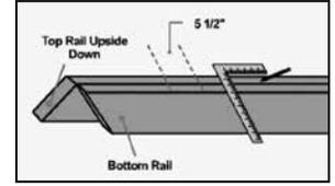
Step 8: Clamp the top and bottom rails together with the top 2x4 rail inverted. Position rails as shown and mark 5-1/2" on-center, working from the center out to the ends of the rails.
