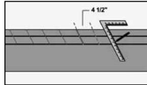
Step 2: Cut top and bottom rails (2x4s) to length and clamp together. Mark top and bottom rails 4-1/2" on-center, starting from the center of the rail.
