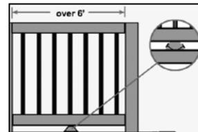
Step 6: For rail sections longer than 4', support blocks are recommended. These can be made from leftover 2x4 rail material. Properly position the support block and toe-nail it to the bottom rail and deck board.
