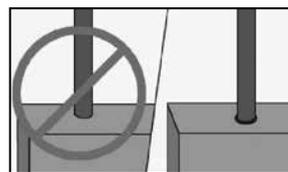
Step 3: Using a drill driver, screw on DecoRators baluster connectors (sold separately) on each mark using the screws provided. Apply silicone caulk on each connector to prevent balusters from turning or rattling after installation is complete. The caulk should be on the outside of the connector, where the baluster will make contact with the connector's outer edge.
