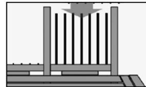
Step 4: Place the bottom rail between the rail posts, supported by a 3" block (2x4 scrap material works best). Secure rail to posts using DecoRators rail connectors (sold separately) and slide balusters over the bottom connectors. Carefully place top rail over the balusters, making sure each baluster is seated properly on each connector.
