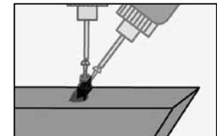
Step 9: Properly position the connectors on the rails. The top and bottom connectors will be facing opposite directions. Screw the connectors in place. To properly set angled connectors, begin screwing vertically until the screw bites into the wood. Reposition screw to the proper angle and tighten. Do not over-tighten, which can move the connector off center.
