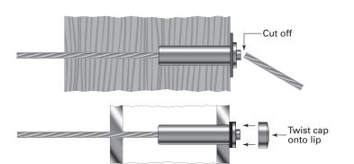
**4.** Twist the cap onto the lip of the Pull-Lock® fitting.
