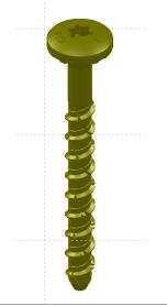
Dimensions are in inches without any manufacturing tollerances! More technical info also avilable under ICC ESR # 3251 Predrilling with a 1/4 inch diameter concrete drill bit requiered. Has a T-40 Star drive.
