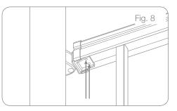
Install pyramid post top onto each post. Note: A rubber mallet may be needed for proper fit.
