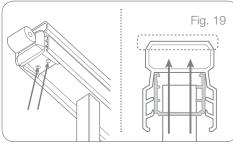
Press top rail end covers onto both ends of
