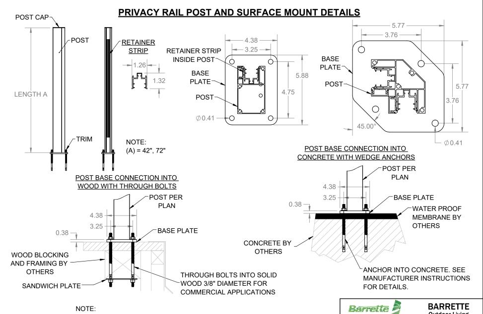
1. COMMERCIAL APPLICATIONS ARE ALWAYS BOLTED, USE 3/8" DIAMETER A307 THROUGH BOLTS INTO SOLID WOOD BLOCKING.
