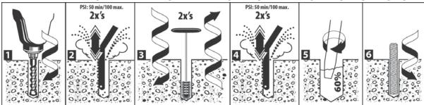
\* Water-saturated concrete, water-filled holes and submerged concrete applications require 4x's air, 4x's brushing and 4x's air
