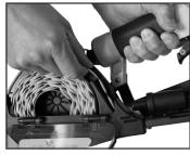
• Place cap reel in the Magazine - make sure the front end of the cap coil is placed over the cap guide area of the Magazine. Insert lead cap into the Feed Chute. Close the Magazine Cover.
