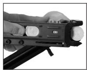
• Slide caps along the Feed Chute with fingers until they engage the Cap Feeder. Pull the Cap Feeder back and release to advance the caps until the first cap is under the Nose of the tool.
