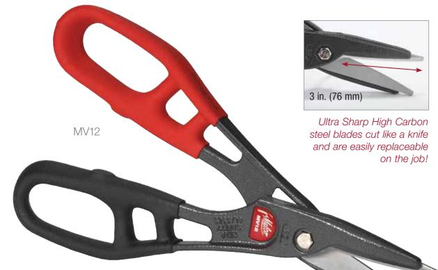
Lightweight 12 in. (31 cm) aluminum handled combination snip, features a BIG 3 in. (76 mm) cutting depth. Inset steel blades feature a Knife like edge that produces a smooth slicing action for cutting thick or layered vinyl and a variety of other flexible <u>non-ferrous</u> materials.
