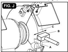
The Wheel Dresser is to be used on the grinding wheels. It will remove buildup up of material on the grinding wheel, remove imperfections and make the corners of the grinding wheel square. See Figure J.
