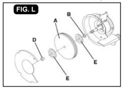
A wire wheel or buffing wheel (A) (not included) can be used with your grinder. Depending on the thickness of the wheel, you will need to add one or more spacers (not included) to allow the arbor hex nut (D) to tighten correctly. Figure L shows the correct placement of the spacer (B).
