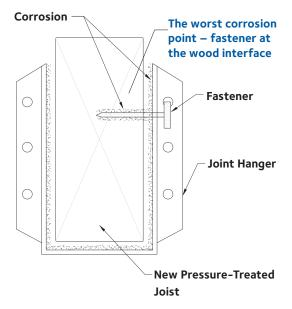
Galvanized joist hanger attached to ACQ wood, 7 months; wet conditions.
