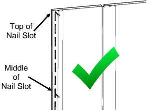
The uppermost nail should be in the top of nail slot on vertical siding. All other nails should be centered in the slot.
