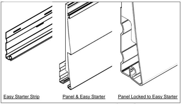
Horizontal siding can be started using the Easy Starter Strip shown above.
