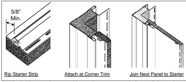
Vertical siding can be started by cutting a starter strip from a full panel and attaching the starter at the 4" (1-1/8" receiver) corner trim.
