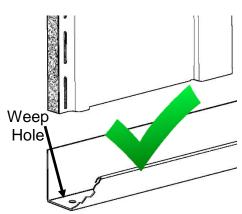
Follow good weatherproofing practices (i.e. drill weep holes in bottom of J-channels)
