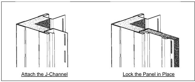
Vertical siding can be started and/or ended using a 3/4" J-Channel.
